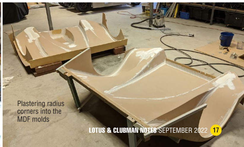
MDF molds being built over the car
