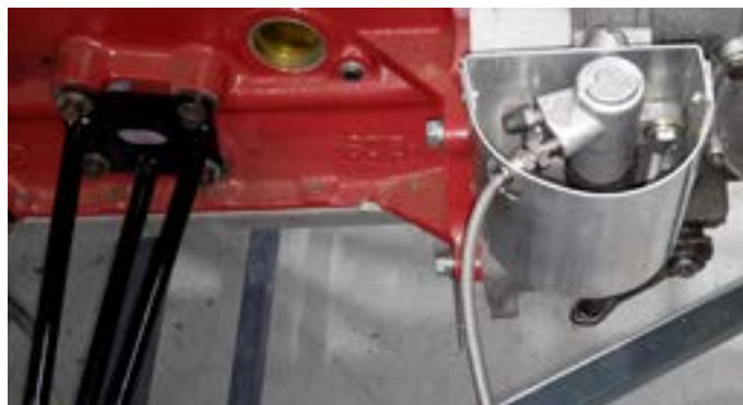
Front Engine Mount (and heat-shielded clutch slave cylinder)
