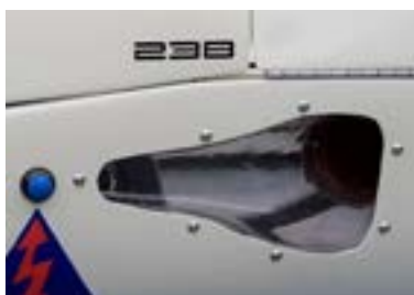
NACA duct channels air to the Oil Cooler
