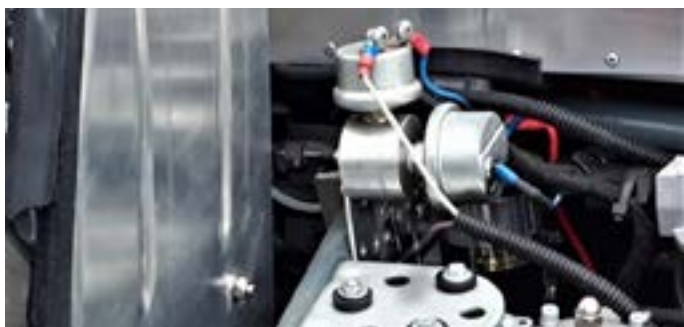
Loss of oil pressure electrical cut-off switch (and oil pressure warning light sender) mounted remotely from engine to avoid vibration failure
