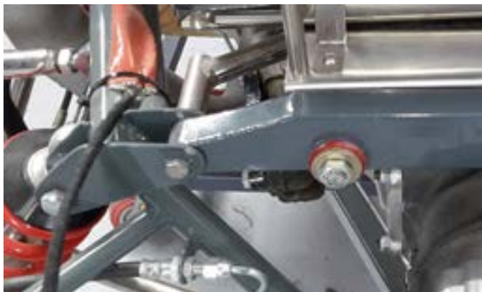
Rear transaxle to chassis mount points
