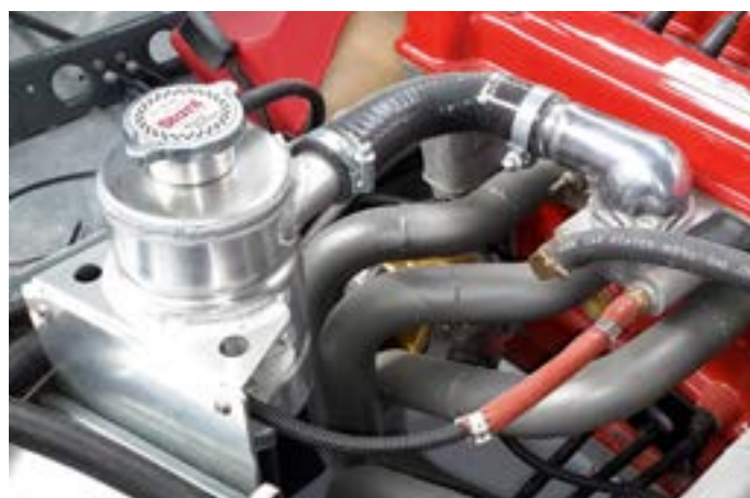
Cooling system Swirl Pot and ceramic coated headers
