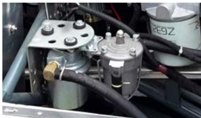
Carter fuel pump with Malpassi filter/pressure regulator
