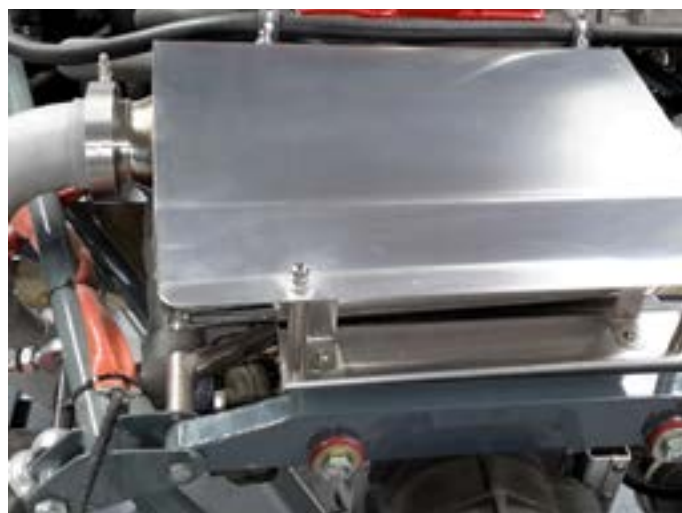
Muffler – protected by "Zircoflex Gold" lined heat shield
