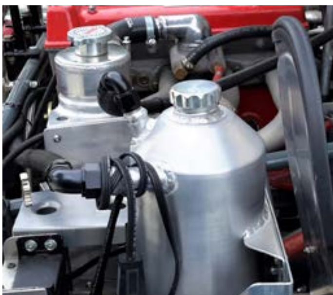
Dry sump system oil tank – note cord for the in-tank heater
