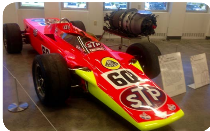
Lotus Type 56 – Pratt & Whitney gas turbine four wheel drive. Four were built.
