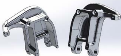
CAD model illustrating two halves of new gearbox mount.
