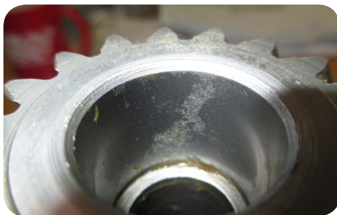
▲ cluster gear corrosion on bearing surface
