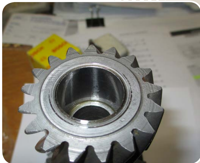
▲ cluster gear new bearing sleeve inserted
