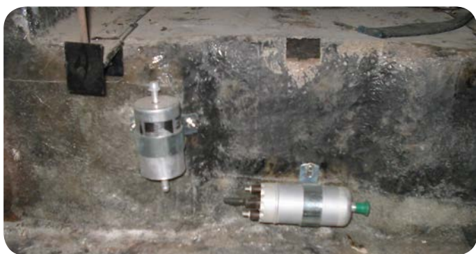
This is an earlier photo taken when the pump, filter and tank straps were trial fitted.
