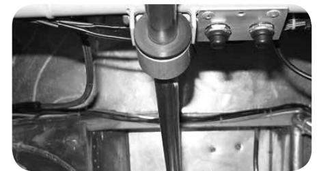
Two pushbuttons by the steering column operate the tattletale function of the Stack electronic tachometer.
