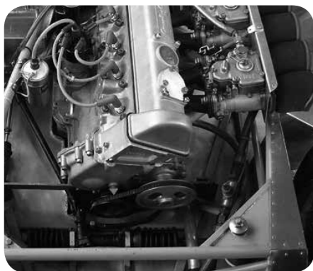
1460cc Coventry Climax (#FWB400-55), rebuilt by Brian MacEachern.
