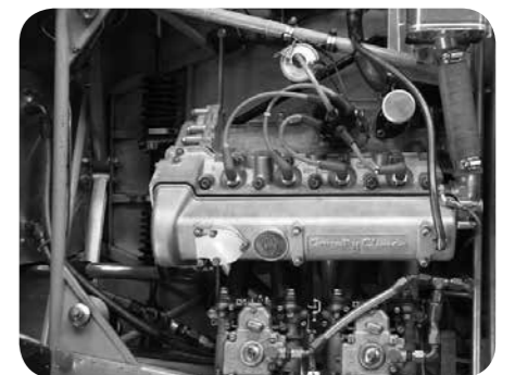
Lotus canted the Coventry Climax engine ten degrees to achieve the lowest feasible bonnet height.
