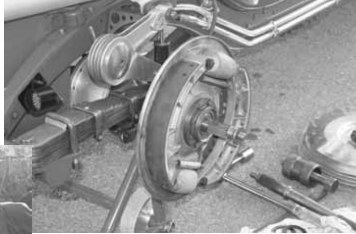
Remember drum brakes? These were on a 1934 Alfa GP car
