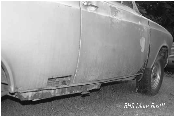
RHS Sill guard rust removed
