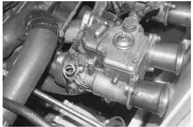
Note wire repairs to weber
